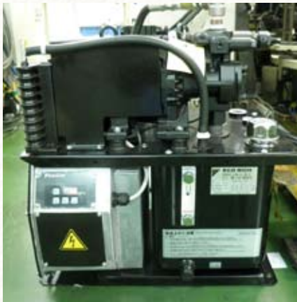
Fujiyama Works Hydraulic pump for cooling fan blade assembly line
